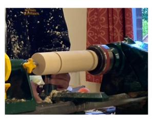
Viv started with 2 3/4" x 2 3/4" redwood and turned between centres until round also creating spigot for mounting in the chuck. No sanding or sealing required as the piece are burned to finish. mounted Once in chuck measure and mark 1/3 to 2/3 leaving some for parting off.
