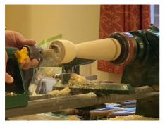
Mark the base and candle cup heights and then form the desired shape, you can add rings etc. Don't make the piece too thin around the neck as it will be burned. Drill hole for candle with Forstner bit.
